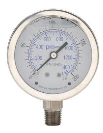
ProSense mechanical pressure gauge, 2.5in diameter, 0 to 200 psig/0 to 1400 kPa, stainless steel liquid filled case, stainless steel wetted parts, 1/4in male NPT process connection, lower mount.
