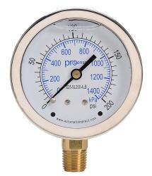
ProSense mechanical pressure gauge, 2.5in diameter, 0 to 200 psig/0 to 1400 kPa, stainless steel liquid filled case, brass wetted parts, 1/4in male NPT process connection, lower mount.
