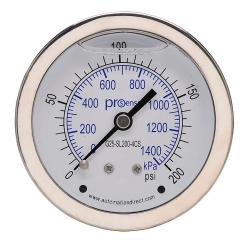
ProSense mechanical pressure gauge, 2.5in diameter, 0 to 200 psig/0 to 1400 kPa, stainless steel liquid filled case, stainless steel wetted parts, 1/4in male NPT process connection, center back mount.
