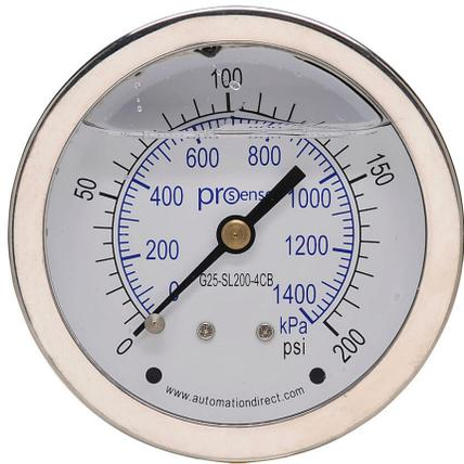
ProSense mechanical pressure gauge, 2.5in diameter, 0 to 200 psig/0 to 1400 kPa, stainless steel liquid filled case, brass wetted parts, 1/4in male NPT process connection, center back mount.
