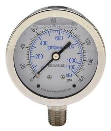
ProSense mechanical pressure gauge, 2.5in diameter, 0 to 160 psig/0 to 1100 kPa, stainless steel liquid filled case, stainless steel wetted parts, 1/4in male NPT process connection, lower mount.
