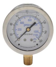
ProSense mechanical pressure gauge, 2.5in diameter, 0 to 160 psig/0 to 1100 kPa, stainless steel liquid filled case, brass wetted parts, 1/4in male NPT process connection, lower mount.
