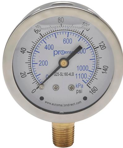
ProSense mechanical pressure gauge, 2.5in diameter, 0 to 160 psig/0 to 1100 kPa, stainless steel liquid filled case, brass wetted parts, 1/4in male NPT process connection, lower mount.
