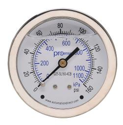
ProSense mechanical pressure gauge, 2.5in diameter, 0 to 160 psig/0 to 1100 kPa, stainless steel liquid filled case, brass wetted parts, 1/4in male NPT process connection, center back mount.
