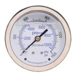
ProSense mechanical pressure gauge, 2.5in diameter, 0 to 1500 psig/0 to 10000 kPa, stainless steel liquid filled case, brass wetted parts, 1/4in male NPT process connection, center back mount.
