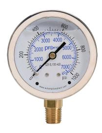
ProSense mechanical pressure gauge, 2.5in diameter, 0 to 1000 psig/0 to 7000 kPa, stainless steel liquid filled case, brass wetted parts, 1/4in male NPT process connection, lower mount.
