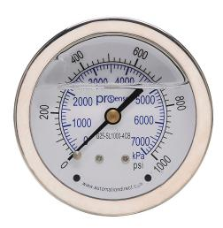
ProSense mechanical pressure gauge, 2.5in diameter, 0 to 1000 psig/0 to 7000 kPa, stainless steel liquid filled case, brass wetted parts, 1/4in male NPT process connection, center back mount.
