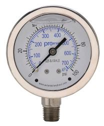
ProSense mechanical pressure gauge, 2.5in diameter, 0 to 100 psig/0 to 700 kPa, stainless steel liquid filled case, stainless steel wetted parts, 1/4in male NPT process connection, lower mount.
