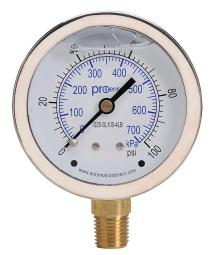
ProSense mechanical pressure gauge, 2.5in diameter, 0 to 100 psig/0 to 700 kPa, stainless steel liquid filled case, brass wetted parts, 1/4in male NPT process connection, lower mount.
