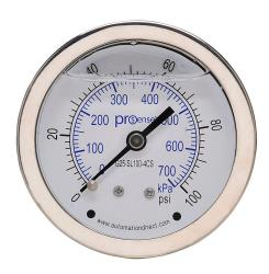
ProSense mechanical pressure gauge, 2.5in diameter, 0 to 100 psig/0 to 700 kPa, stainless steel liquid filled case, stainless steel wetted parts, 1/4in male NPT process connection, center back mount.
