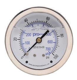
ProSense mechanical pressure gauge, 2.5in diameter, 0 to 100 psig/0 to 700 kPa, stainless steel liquid filled case, brass wetted parts, 1/4in male NPT process connection, center back mount.
