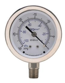
ProSense mechanical pressure gauge, 2.5in diameter, -30 to 0in Hg vacuum/-100 to 0 kPa, stainless steel dry case, stainless steel wetted parts, 1/4in male NPT process connection, lower mount.
