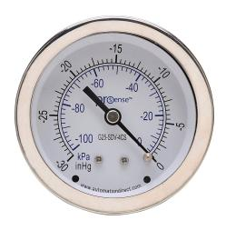
ProSense mechanical pressure gauge, 2.5in diameter, -30 to 0in Hg vacuum/-100 to 0 kPa, stainless steel dry case, stainless steel wetted parts, 1/4in male NPT process connection, center back mount.
