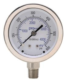
ProSense mechanical pressure gauge, 2.5in diameter, 0 to 600 psig/0 to 4200 kPa, stainless steel dry case, stainless steel wetted parts, 1/4in male NPT process connection, lower mount.
