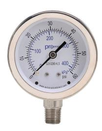
ProSense mechanical pressure gauge, 2.5in diameter, 0 to 60 psig/0 to 420 kPa, stainless steel dry case, stainless steel wetted parts, 1/4in male NPT process connection, lower mount.
