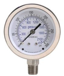
ProSense mechanical pressure gauge, 2.5in diameter, 0 to 300 psig/0 to 2100 kPa, stainless steel dry case, stainless steel wetted parts, 1/4in male NPT process connection, lower mount.
