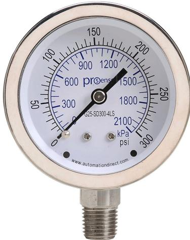
ProSense mechanical pressure gauge, 2.5in diameter, 0 to 300 psig/0 to 2100 kPa, stainless steel dry case, stainless steel wetted parts, 1/4in male NPT process connection, lower mount.
