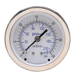
ProSense mechanical pressure gauge, 2.5in diameter, 0 to 30 psig/0 to 210 kPa, stainless steel dry case, stainless steel wetted parts, 1/4in male NPT process connection, center back mount.
