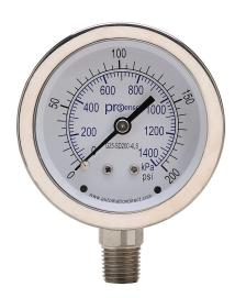
ProSense mechanical pressure gauge, 2.5in diameter, 0 to 200 psig/0 to 1400 kPa, stainless steel dry case, stainless steel wetted parts, 1/4in male NPT process connection, lower mount.
