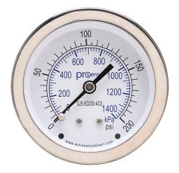
ProSense mechanical pressure gauge, 2.5in diameter, 0 to 200 psig/0 to 1400 kPa, stainless steel dry case, stainless steel wetted parts, 1/4in male NPT process connection, center back mount.
