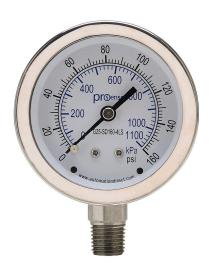
ProSense mechanical pressure gauge, 2.5in diameter, 0 to 160 psig/0 to 1100 kPa, stainless steel dry case, stainless steel wetted parts, 1/4in male NPT process connection, lower mount.
