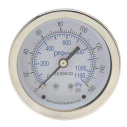
ProSense mechanical pressure gauge, 2.5in diameter, 0 to 160 psig/0 to 1100 kPa, stainless steel dry case, stainless steel wetted parts, 1/4in male NPT process connection, center back mount.
