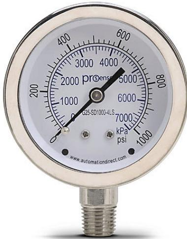
ProSense mechanical pressure gauge, 2.5in diameter, 0 to 1000 psig/0 to 7000 kPa, stainless steel dry case, stainless steel wetted parts, 1/4in male NPT process connection, lower mount.
