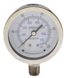
ProSense mechanical pressure gauge, 2.5in diameter, 0 to 100 psig/0 to 700 kPa, stainless steel dry case, stainless steel wetted parts, 1/4in male NPT process connection, lower mount.
