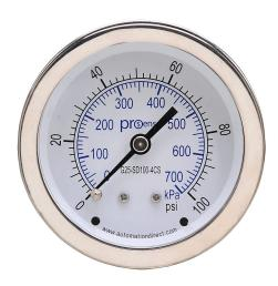
ProSense mechanical pressure gauge, 2.5in diameter, 0 to 100 psig/0 to 700 kPa, stainless steel dry case, stainless steel wetted parts, 1/4in male NPT process connection, center back mount.
