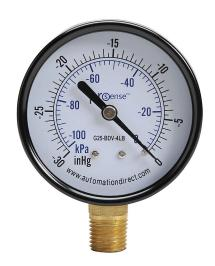
ProSense mechanical pressure gauge, 2.5in diameter, -30 to 0in Hg vacuum/-100 to 0 kPa, black steel dry case, brass wetted parts, 1/4in male NPT process connection, lower mount.
