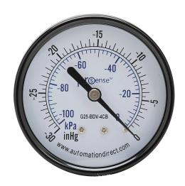
ProSense mechanical pressure gauge, 2.5in diameter, -30 to 0in Hg vacuum/-100 to 0 kPa, black steel dry case, brass wetted parts, 1/4in male NPT process connection, center back mount.
