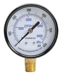
ProSense mechanical pressure gauge, 2.5in diameter, 0 to 600 psig/0 to 4000 kPa, black steel dry case, brass wetted parts, 1/4in male NPT process connection, lower mount.
