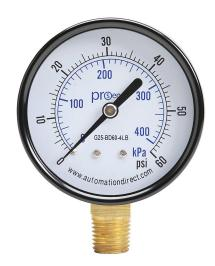
ProSense mechanical pressure gauge, 2.5in diameter, 0 to 60 psig/0 to 400 kPa, black steel dry case, brass wetted parts, 1/4in male NPT process connection, lower mount.
