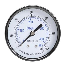
ProSense mechanical pressure gauge, 2.5in diameter, 0 to 60 psig/0 to 400 kPa, black steel dry case, brass wetted parts, 1/4in male NPT process connection, center back mount.
