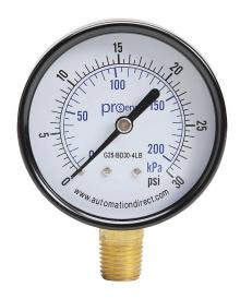
ProSense mechanical pressure gauge, 2.5in diameter, 0 to 30 psig/0 to 200 kPa, black steel dry case, brass wetted parts, 1/4in male NPT process connection, lower mount.
