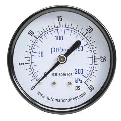
ProSense mechanical pressure gauge, 2.5in diameter, 0 to 30 psig/0 to 200 kPa, black steel dry case, brass wetted parts, 1/4in male NPT process connection, center back mount.
