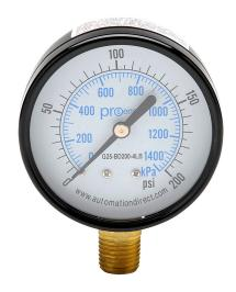
ProSense mechanical pressure gauge, 2.5in diameter, 0 to 200 psig/0 to 1400 kPa, black steel dry case, brass wetted parts, 1/4in male NPT process connection, lower mount.
