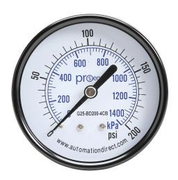
ProSense mechanical pressure gauge, 2.5in diameter, 0 to 200 psig/0 to 1400 kPa, black steel dry case, brass wetted parts, 1/4in male NPT process connection, center back mount.
