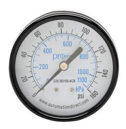
ProSense mechanical pressure gauge, 2.5in diameter, 0 to 160 psig/0 to 1100 kPa, black steel dry case, brass wetted parts, 1/4in male NPT process connection, center back mount.
