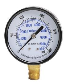
ProSense mechanical pressure gauge, 2.5in diameter, 0 to 1000 psig/0 to 7000 kPa, black steel dry case, brass wetted parts, 1/4in male NPT process connection, lower mount.
