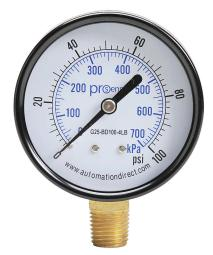
ProSense mechanical pressure gauge, 2.5in diameter, 0 to 100 psig/0 to 700 kPa, black steel dry case, brass wetted parts, 1/4in male NPT process connection, lower mount.
