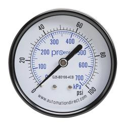
ProSense mechanical pressure gauge, 2.5in diameter, 0 to 100 psig/0 to 700 kPa, black steel dry case, brass wetted parts, 1/4in male NPT process connection, center back mount.
