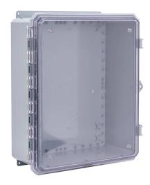
Integra Genesis series enclosure, NEMA 1/2/3/3R/3S/4/4X/5/6/6P/12/13, 20 x 16 x 8in (HxWxD), wall mount, polycarbonate, gray, gloss finish, clear polycarbonate single-door, glass-filled nylon quick-release latch, padlock hasp and staple.
