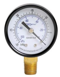
ProSense mechanical pressure gauge, 2in diameter, -30 to 0in Hg vacuum/-100 to 0 kPa, black steel dry case, brass wetted parts, 1/4in male NPT process connection, lower mount.
