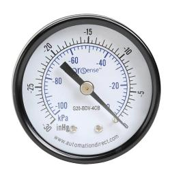
ProSense mechanical pressure gauge, 2in diameter, -30 to 0in Hg vacuum/-100 to 0 kPa, black steel dry case, brass wetted parts, 1/4in male NPT process connection, center back mount.
