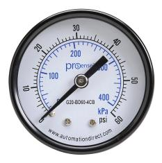
ProSense mechanical pressure gauge, 2in diameter, 0 to 60 psig/0 to 400 kPa, black steel dry case, brass wetted parts, 1/4in male NPT process connection, center back mount.
