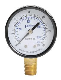
ProSense mechanical pressure gauge, 2in diameter, 0 to 30 psig/0 to 200 kPa, black steel dry case, brass wetted parts, 1/4in male NPT process connection, lower mount.
