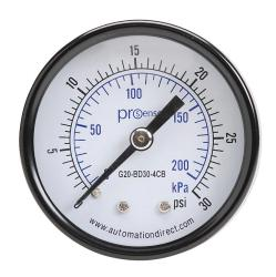
ProSense mechanical pressure gauge, 2in diameter, 0 to 30 psig/0 to 200 kPa, black steel dry case, brass wetted parts, 1/4in male NPT process connection, center back mount.
