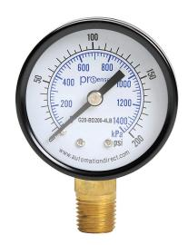
ProSense mechanical pressure gauge, 2in diameter, 0 to 200 psig/0 to 1400 kPa, black steel dry case, brass wetted parts, 1/4in male NPT process connection, lower mount.
