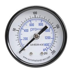
ProSense mechanical pressure gauge, 2in diameter, 0 to 200 psig/0 to 1400 kPa, black steel dry case, brass wetted parts, 1/4in male NPT process connection, center back mount.
