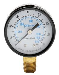
ProSense mechanical pressure gauge, 2in diameter, 0 to 160 psig/0 to 1100 kPa, black steel dry case, brass wetted parts, 1/4in male NPT process connection, lower mount.
