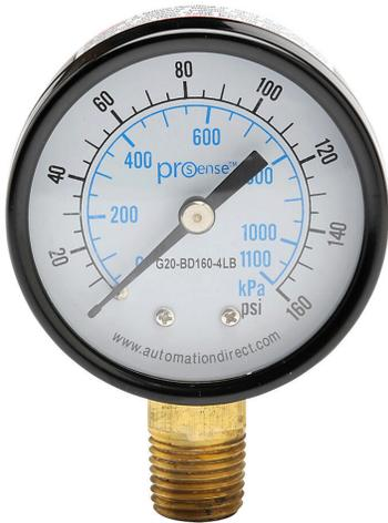
ProSense mechanical pressure gauge, 2in diameter, 0 to 160 psig/0 to 1100 kPa, black steel dry case, brass wetted parts, 1/4in male NPT process connection, lower mount.
