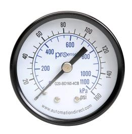
ProSense mechanical pressure gauge, 2in diameter, 0 to 160 psig/0 to 1100 kPa, black steel dry case, brass wetted parts, 1/4in male NPT process connection, center back mount.
